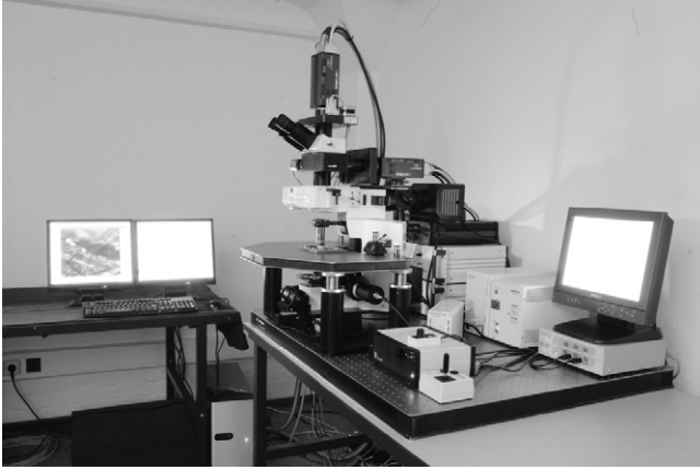
FIG. 2. Side view of a modern intravital microscope. The upright microscope is mounted onto a motorized xy stage that is placed on a stable desk. Several light sources and detectors are connected to the system enabling video and/or digital recording of experiments. Filters and dichroic mirrors can be inserted at different positions in the illumination and detection pathways providing a versatile system that allows a whole variety of different microscopy techniques and experiments (Courtesy LaVision BioTec, Bielefeld, Germany.)
