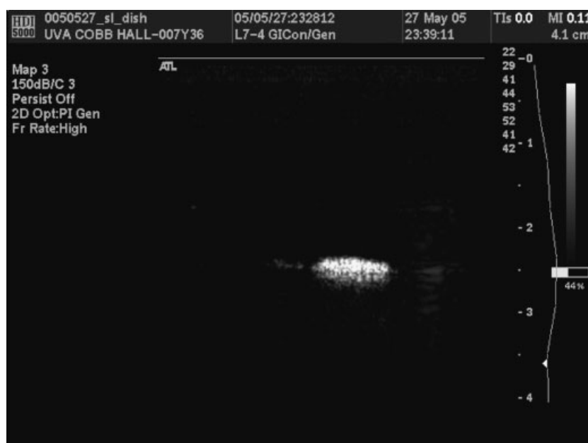
Figure 5. Ultrasound imaging of PSLe x -targeted bubbles on the 35 mm petri dish with P-selectin coated spot in the center. Imaging performed with an HDI5000 system in the general pulse inversion mode at MI \approx 0.1.
